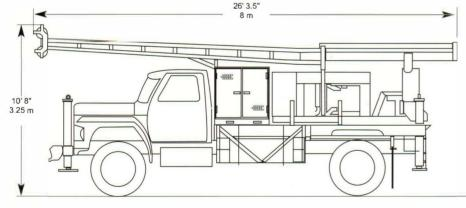
Typical single rear axle truck configuration with 26' mast and optional deck platform. Dimensions will vary, depending on truck wheel base and all-wheel drive or tandem rear axle applications.
